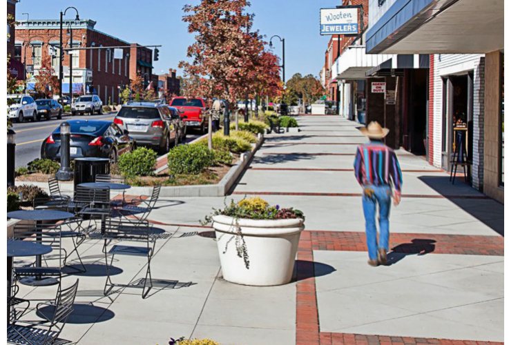
Figure 6.1: Sidewalks shall have clear pedestrian routes of travel and no furnishings within 30 inches of back of curb.
