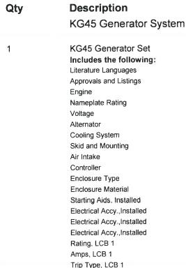
English UL2200 Listing/cUL Genset List SnglFuel, PreAlarm,NG,Stdby Standby 130C Rise 60Hz. 120/240V. 1Ph. 3W 4Q7BX, 1Ph Unit Mounted Radiator, 50C Skid, 41" Standard Duty APM402 Sound Steel 1500W,120V Battery, 1/12V, Wet Battery Charger, 10A 2 Input/5 OutputModule 100% Rated 200 Thermal Magnetic
