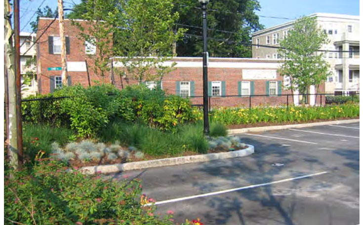
Figure 6.6: Buffered surface parking lot with mounded planting areas for additional headlight buffering.
